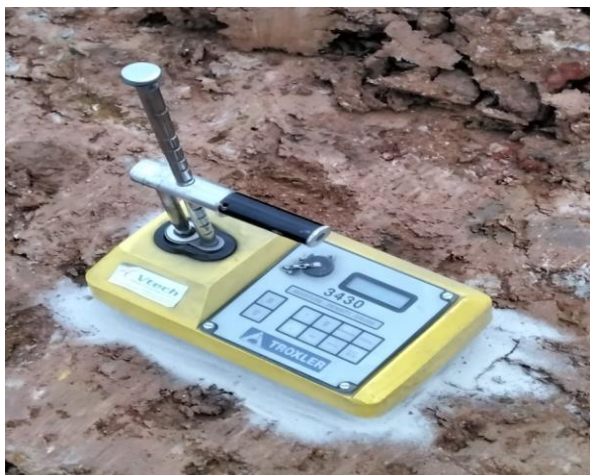
Photo 9: Field density/moisture test
